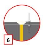
Sand must be at least 1/8" lower than the top of the surface.
