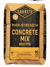
Sakrete® High Strength Concrete Mix is a preblended mixture of sand, coarse aggregate, and cementitious materials. For new construction or repairs where concrete thickness exceeds 2" (51 mm).
