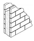
California Building Code (CBC) Sections 2105.1 and 2105A.1 refer to TMS 602 for compliance with the specified  $f'_m$  value. One of two methods must be used (not both): 1) unit strength method or 2) prism test method.
