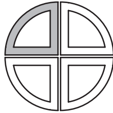
Radius ends cut from 8x8x16 unit.
