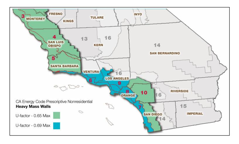
Figure 1 – Southern California Climate Zones with Concrete Masonry Heavy Mass Wall Overlay
