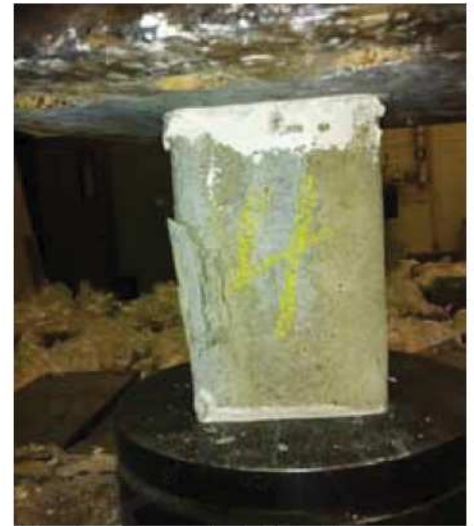
Figure 3: Grout samples during testing.
