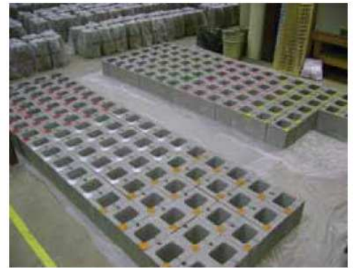
Figure 1: Concrete masonry units prior to casting grout samples.
