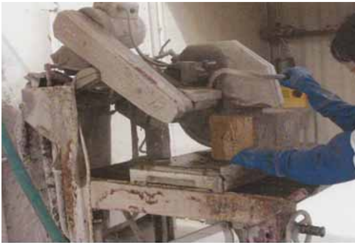
Figure 2: Test Specimens Being Saw-Cut From Concrete Masonry Unit Cells
