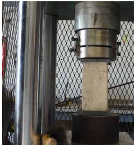
Figure 3: Compression Testing of Grout Specimen
