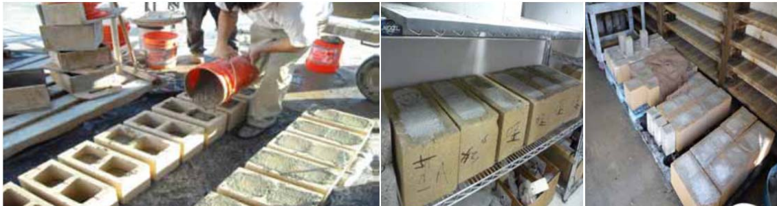
Figure 1: Grout Placement and Dry and Wet Curing of Specimens
